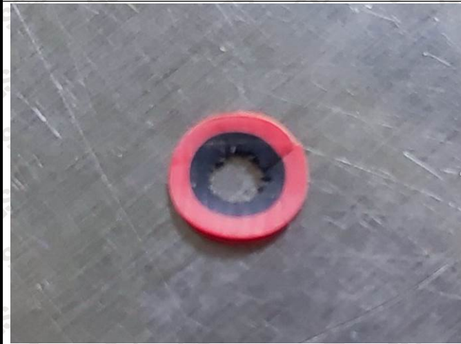
Dimension check-Thickness of jacket and insulation
